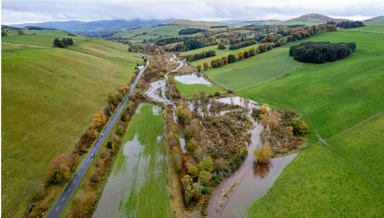
Re-meandering of Eddleston Water in the Tweed catchment © Colin MacLean
